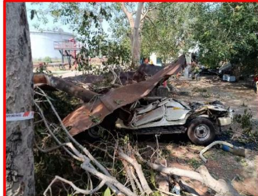
Figure 2: Dome of the second exploded tank.
