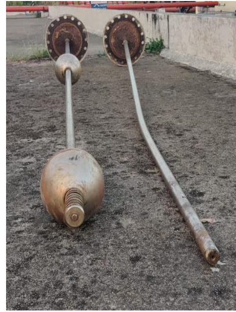
LEFT (MAGNETIC LEVEL GAUGE) RIGHT (DEFECTIVE MAGNETIC LEVEL GAUGE)
