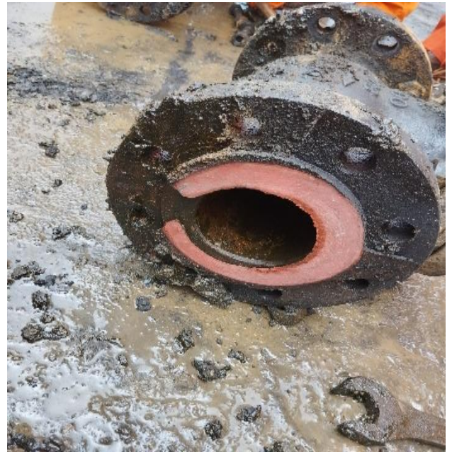
Questioned gasket which gave way.
