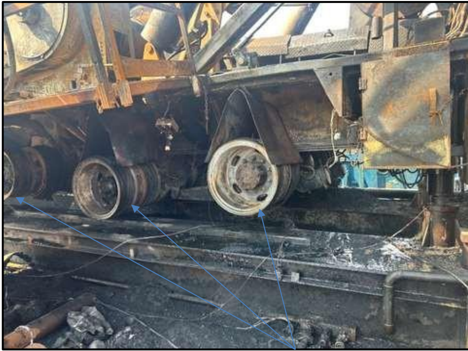
12 rear tyres (Including both side) completely burnt
