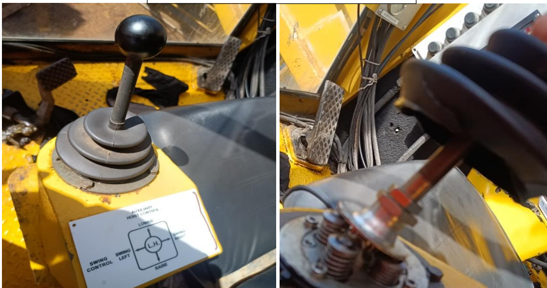
Figure II – Dual-joystick control system of crane
