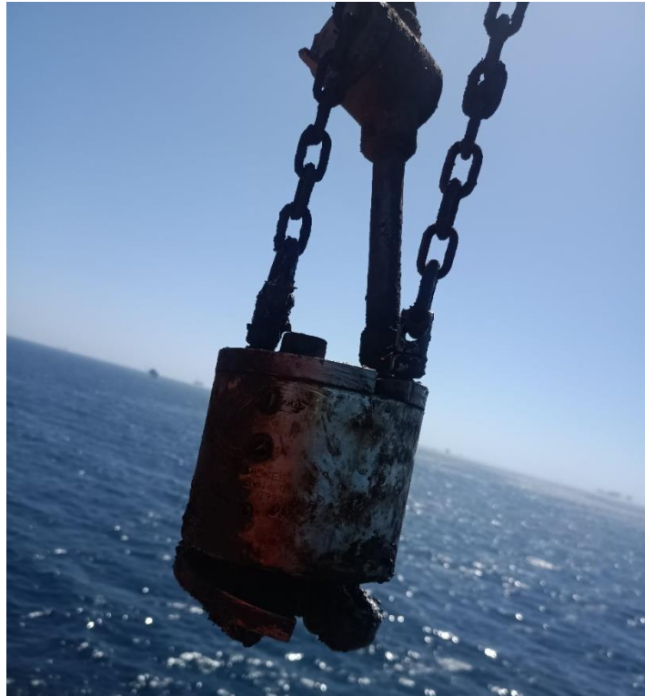
Figure III – Main Anti-Two Block
